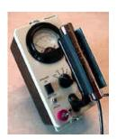
Scintillation instruments use light produced by the interaction of radiation with a light-producing material (liquid or solid) to detect radiation. The amount of light during an interaction is proportional to the energy of radiation. Photomultiplier tubes and multichannel analyzers are often employed with scintillation instruments in order energy-discriminate and produce qualitative and quantitative spectra.
