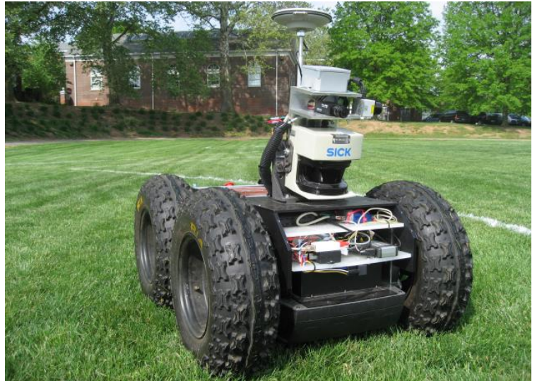
Warthog robot made by University of Delaware, IGVC 2008
