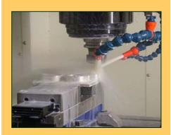
Only a few millilitres of coolant sufficient for long tool life.
