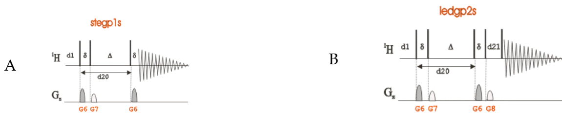
Figure 6. (A) The stimulated echo (STE) DOSY pulse sequence differs from the gradient spin echo in that the 180^\circ pulse has been replaced by 2 90^\circ pulses, the result is that magnetization is moved back to the z axis after first gradient pulse where it undergoes T1 relaxation during the long delay \Delta that is slower than the T2 relaxation experienced by magnetization in the xy plane. This results in a greater signal to noise ratio for this experiment. (B) The longitudinal eddy current delay (LED) pulse sequence. This sequence is a further modification of the STE sequence that has an extra delay (d21) inserted between the last gradient and the beginning of the signal acquisition to allow any eddy currents developed by the gradients pulses to decay before acquisition begins.
