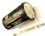
Fig. 1(b) Battery to wire connection secured with tape
