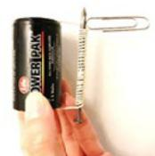
Fig. 1(c) Electromagnet testing: magnet holding paper clip
