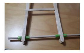
iii. Make sure the dowel can freely spin in both straws.
