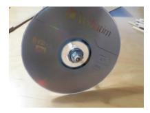
v. Glue a wheel on each side of the dowel. Be sure to avoid gluing the wheels to the straw.
