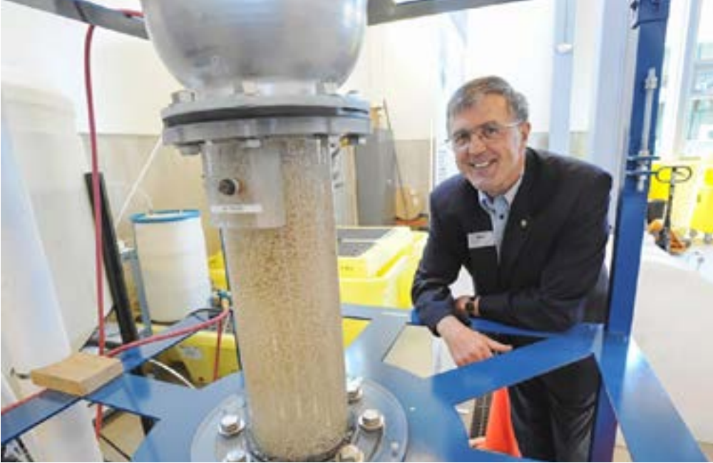
Don Mavinic poses in front of his research team's fourth-generation crystal reactor demo unit run by Metro Vancouver at the Annacis Research Centre on Annacis Island, BC. (Photo courtesy of the University of British Columbia)
