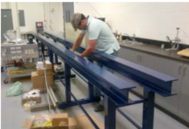
Luigi Zanettin works on a Hopkinson’s Split Pressure Bar Apparatus he helped design and build at the Ed Lumley Centre for Engineering Innovation.
