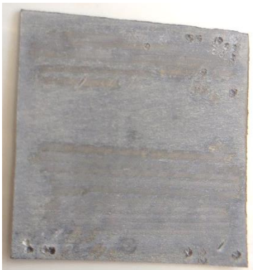
Figure 4.3: A camera picture of the neodymium platelet used as the target for both single and dual pulse LIBS experiments.
