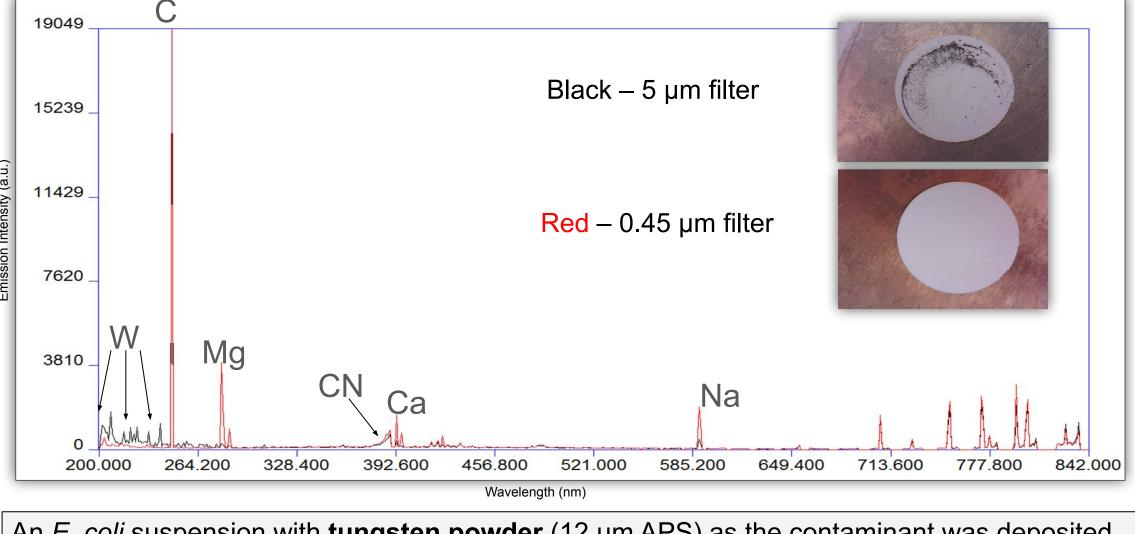
An *E. coli* suspension with **tungsten powder** (12 µm APS) as the contaminant was deposited in the insert with the 5 µm filter paper on top and the 0.45 µm filter paper below it. The tungsten powder was caught by the 5 µm filter while ~ 90% of the bacteria passed through it and settled onto the 0.45 µm filter.
