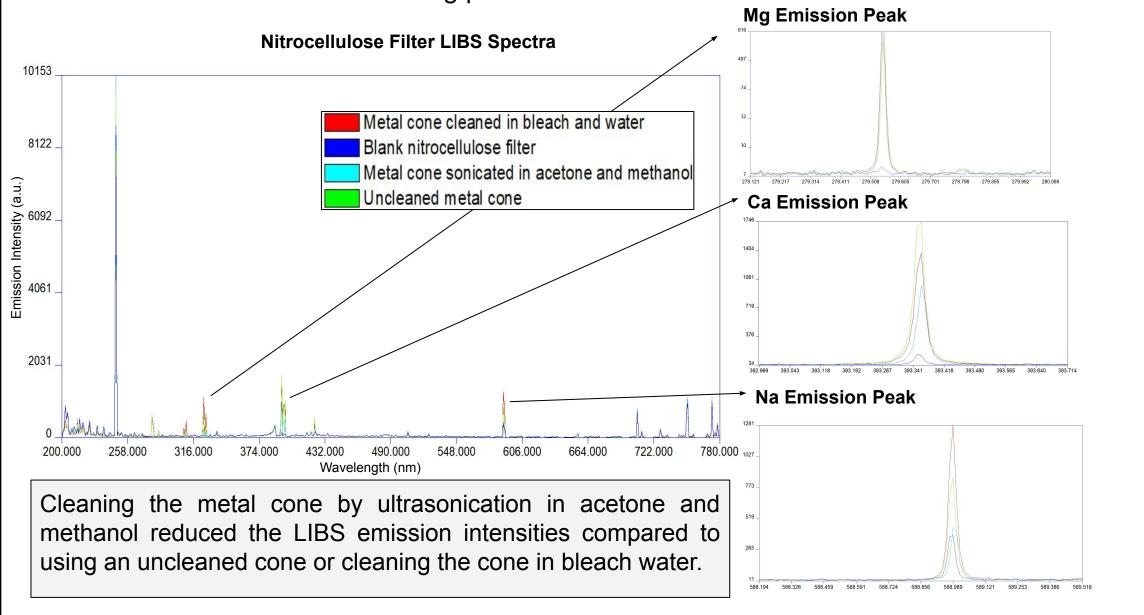
**Conclusion:** Cleaning the metal cone with an appropriate procedure yielded a significant reduction in the emission peak intensities in the absence of bacteria.
