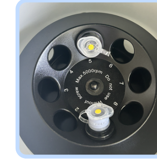
Sample is centrifuged at 2400 rpm for 5 minutes, allowing for aCSF to drain through filter as bacteria are concentrated at centre.
