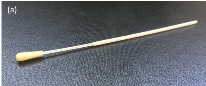
(a) Flocked swab used in this work. (b) Flocked swab zoomed-in on the tip
