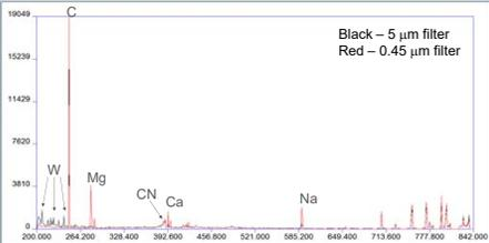
**Conclusion:** The use of this centrifuge tube insert with filter media of different pore sizes was effective at separating a contaminant from bacteria.
