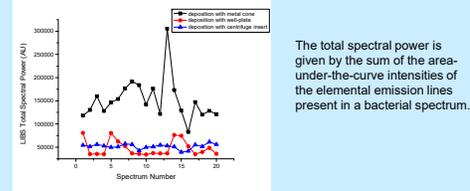
**Conclusion:** The use of the metal cone for deposition on the filter paper as opposed to other deposition methods results in an increased LIBS bacterial signal.
