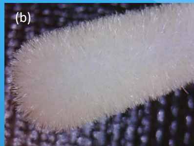
(a) Flocked swab used in this work. (b) Flocked swab zoomed-in on the tip
