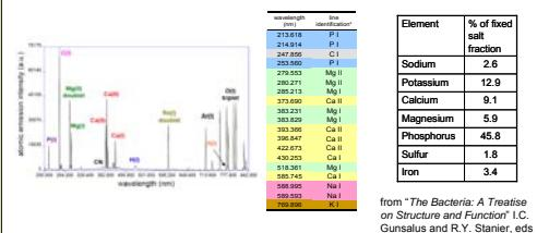
LIBS spectra obtained from bacteria prepared identically over the span of months demonstrate high reproducibility. When classified by EMMA the results are consistent over months/years. This suggests that inherent repeatability is not a limiting factor.
