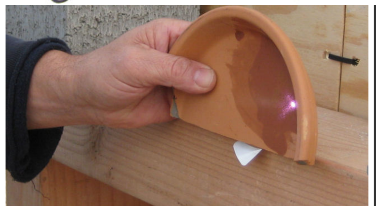
Laser plasma on clay target at 50 metres range (Hidden Valley, NTC, December 2007) (Published with permission of U.S. Army, National Training Center, Fort Irwin) Image 15 of 23
